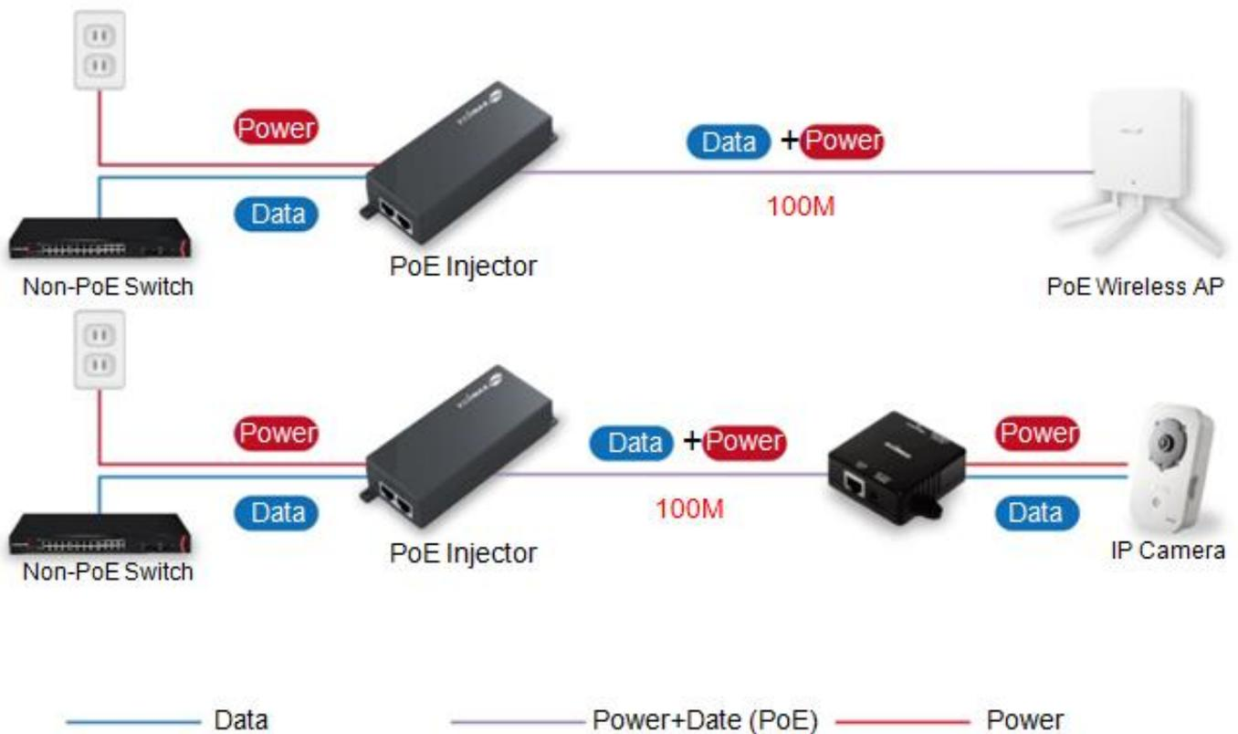
**⚠ The PoE/DATA port sends power and Ethernet data to your PoE-enabled device. Use a CAT 5 cable to connect the PoE/Data port to your PoE-enabled device.**
