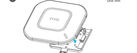
**EN** 1 Attach two clips to the ceiling grids as shown. 2 Install two screws to secure the bracket to the clips. 3 Slide the WAX510D onto the bracket until it clicks into the place. **Note:** Clips (ACCESSORY-ZZ0105F) are sold separately.
