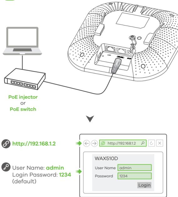
**EN** 1-b Use an Ethernet cable to connect your computer to the **UPLINK** port of the WAX510D through a PoE injector or PoE switch. Use its DHCP-assigned IP or default static IP address "http://192.168.1.2" to access the web configurator. Make sure your computer IP address is in the same subnet as the WAX510D's.
