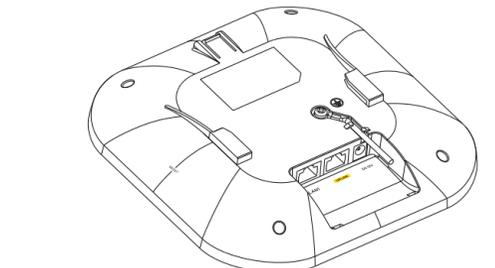
**EN** 1 Remove the M4 ground screw from the WAX510D's rear panel as shown. Secure a green/yellow ground cable (18 AWG or smaller) to the WAX510D's rear panel using the M4 ground screw.
