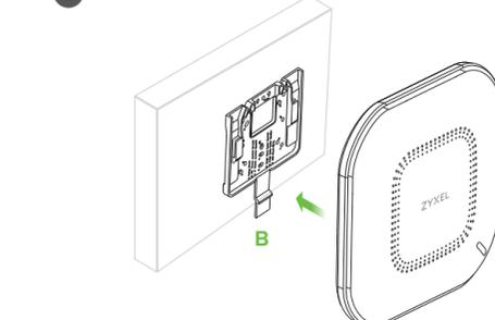
**EN** 2 Install two mounting screws through the holes on the bracket (B) into the plugs/anchors to secure the bracket to the wall/ceiling. Make sure the screws are snugly and securely fastened to the wall/ceiling.
