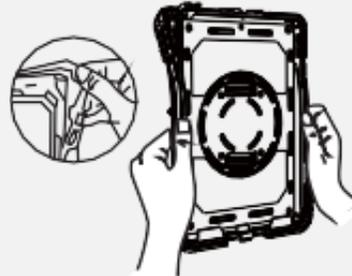
2. Peel the silicone corner shell back on all four corners.
