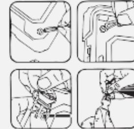
3. The device includes a lanyard strap, the holes found behind the silicone are specifically for this feature. (lanyard not included)
