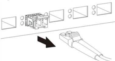
**Figure 17** Opening the Transceiver's Latch Example
