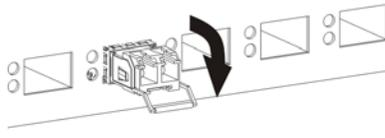
**Figure 18** Transceiver Removal Example
