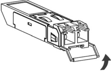
**Figure 14** Transceiver Installation Example
