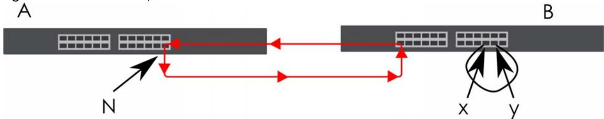
The loop guard feature checks to see if a loop guard enabled port is connected to a Switch in loop state. This is accomplished by periodically sending a probe packet and seeing if the packet returns on the same port. If this is the case, the Switch will shut down the port connected to the switch in loop state.
