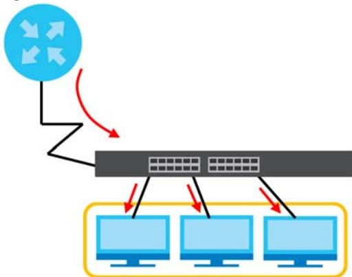
Figure 102 Static Multicast Forwarding to a Single Port
