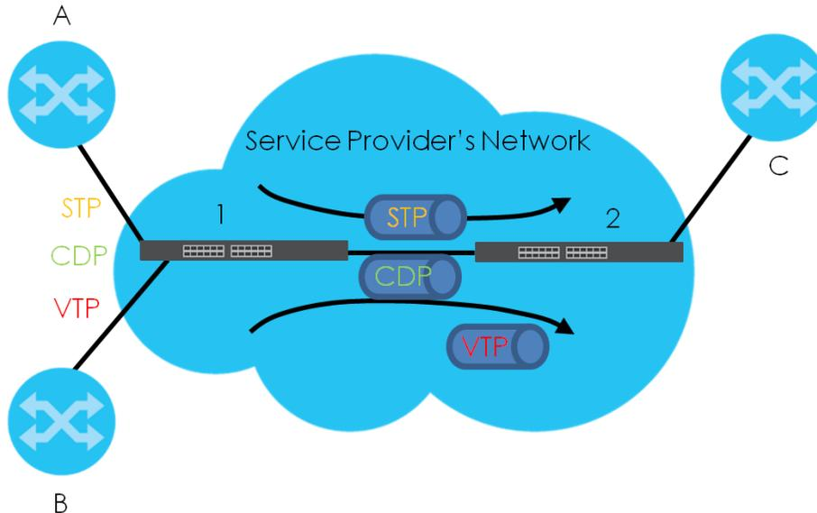
In the following example, if you enable L2PT for STP, you can have switches **A**, **B**, **C** and **D** in the same
