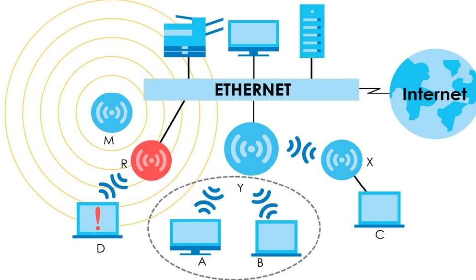
The following figure shows you how to create a secure Wireless Distribution System (WDS). The root AP (Y) is connected to a network with Internet access and has wireless repeaters (X and Z) connected to it to expand the wireless network's range. Clients (A and B) can access the wired network through the wireless repeaters (X and Z) and/or root AP.
