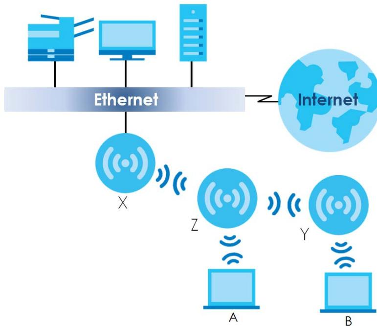
When the Zyxel Device is in Repeater mode, repeater security between the Zyxel Device and other repeater is independent of the security between the wireless clients and the AP or repeater. When repeater security is enabled, both APs and repeaters must use the same pre-shared key. See [Section 10.2 on page 77](#) and [Section 13.2 on page 128](#) for more details.
