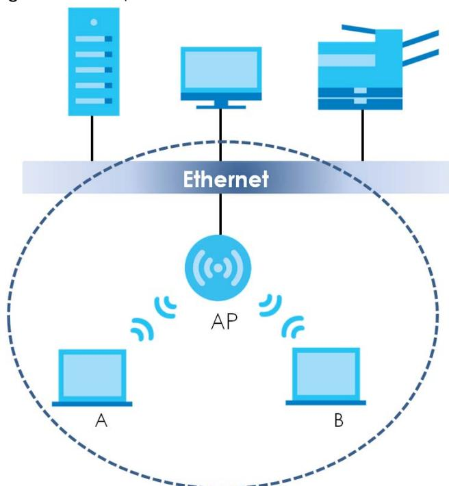
The wireless network is the part in the blue circle. In this wireless network, devices **A** and **B** are called wireless clients. The wireless clients use the access point (AP) to interact with other devices (such as the printer) or with the Internet. Your Zyxel Device is the AP.
