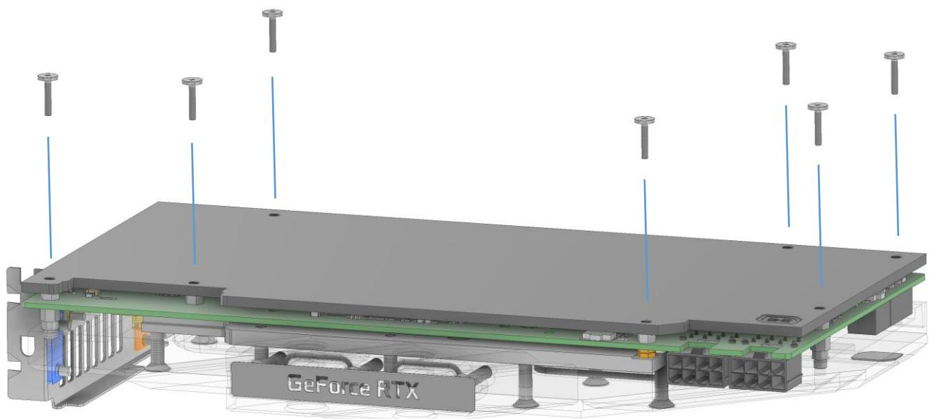
**EN** Put the backplate on and screw it together with the 7 M2x11 screws as shown.
