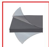
**EN** Remove the protective foils from the thermal pads and place the pads on the PCB as shown.
