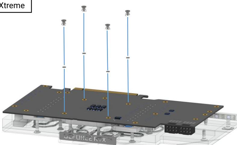
**EN** Place the graphics card on the prepared cooler. Fasten the card as shown with the 4 M2x5 screws with M2 washers. Hand-tighten the screws crosswise, one turn at a time.
