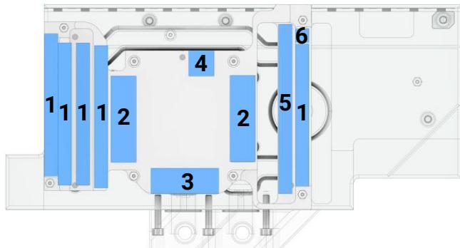
**EN** Clean the contact surfaces on the bottom side of the cooler with alcohol or similar. The surface must be free of contaminants.
