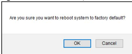
If you want to access the Switch Web Configurator again, you may need to change the IP address of your computer to be in the same subnet as that of the default Switch IP address (192.168.1.1 or DHCP-assigned IP).
