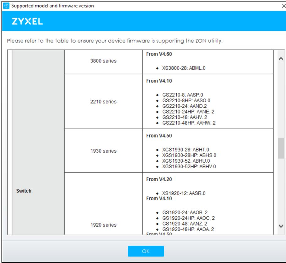
If you want to check the supported models and firmware versions later, you can click the **Show information about ZON** icon in the upper right of the screen. Then select the **Supported model and firmware version** link. If your device is not listed here, see the device release notes for ZON Utility support. The release notes are in the firmware zip file on the ZyXel web site.
