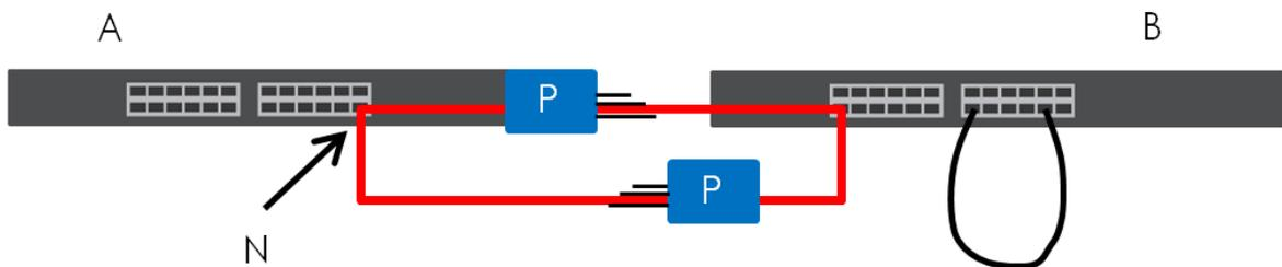
The Switch also shuts down port N if the probe packet returns to switch A on any other port. In other words loop guard also protects against standard network loops.
